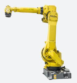
The FANUC M-710iC/50 is battle-ready and one of FANUC's intelligent robots. The robot is coated with a protective epoxy. Its wrist can withstand high-pressure washing. Each joint has extra oil seals and every bolt is coated. The 710 iC 50 can be immersed in 15 cm to 1 m of liquid and is certifiably protected from all dust, cutting down on wear and tear. Even the robot's base is safeguarded, designed to expel air, thus preventing outside air from seeping into the robotic arm.
