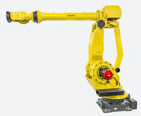
The FANUC M-900iA/260L industrial robot arm features an extended horizontal reach to incorporate larger parts than the standard 900 robot arm. This robot can be floor, angle, or ceiling mounted to further produce a versatile and space savings workspace. Also, the slim, stationary outer arm helps to simplify hose and cable dress out, prolong service life, and also minimize interference with system peripherals in confined spaces.
