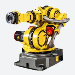
The FANUC R-2000iB/170CF robot can be mounted on the floor or ceiling and can handle payloads up to 170 kg. Perfect for almost all kinds of material handling, as well as spot welding and material removal, the R-2000iB/170CF robot also offers a small footprint, six axes, and an IP67 rated wrist/forearm.
