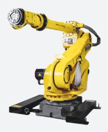
The heavy-duty power of the R-2000iB/185L is able to handle a vast array of high payload applications. With a large work envelope and an extended reach, this productive robot is able to provide manufacturers with the flexibility they require to stay on top of the production game in their market.
