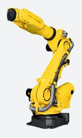
The FANUC R-2000iB/210FS is not only high in flexibility, reach, and payload, but it is also a robot that is able to cut down on maintenance costs over the life of the robot. With high wrist moments and inertia, the R-2000iB/210FS can handle almost any gripper or welding torch, improving cycle times for a variety of applications.
