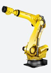
With a payload of 270 kg, the FANUC R-2000iC/270F R-30iB is one of the strongest robots in its class. The R-2000iC/270F is capable of handling a variety of heavy payload applications, including spot welding and palletizing. The FANUC R-2000iC/270F comes equipped with the R30iB controller. If you are looking for a versatile, dependable, strong robot, the FANUC R-2000iC/270F is an excellent choice.
