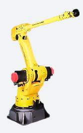
A large work envelope and a 15 kg payload capacity make the FANUC S-500 able to perform a wide variety of industrial applications such as dispensing, material handling, welding, and parts transfer. Multiple mounting options and a slender arm design make the new and used S-500 easy to integrate into any factory floor. The new or reconditioned FANUC S-500 can use the R-J2, R-J3, or the R-J3iB FANUC controllers.
