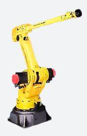
The 6-axis FANUC S-500iB is designed for high-speed smooth movements. The refined movement of the S-500iB R-J3iB, a result of RV speed reducers, is powered by brushless AC servo motors. Cables are routed through hollow joints on the S-500ib arm to reduce interference.
