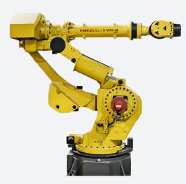
The FANUC S-900iB/400 is a high quality, durable robot that is great for many of your heavy duty application needs. The 400 kg payload capacity is great for lifting a variety of heavy materials, including automobiles, construction materials, tile pallets, and brick pallets.
