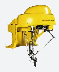
The FANUC M-1iA/0.5A represents one of the fastest, most accurate robots in manufacturing today. Designed for use in pick and place and/or material handling applications, the parallel-link structure allows the M-1iA/0.5A R30iA very fast axis speeds over a 280 millimeter work envelope.
