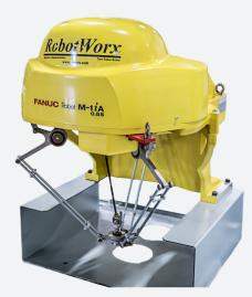
This 4-axis version of the FANUC M-1iA/0.5S Genkotsu (fist) robot can reach speeds up to 3000 degrees per second. This makes the FANUC M-1iA/0.5S R-30iA/R-30iB a first choice for applications with light payloads and speed requirements. It can be installed as a robot only (no stand), as a desktop mount with a stand, at an angle, or on the ceiling. The lightweight design of the M-1iA/0.5S robot makes it flexible for installation in small spaces.
