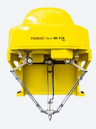
The FANUC M-1iA/1H robot delivers high speed pick and place. The FANUC M1iA/1H has a 1 kg payload and is ideal for applications needing a fast pick and place motion without needing to rotate the parts. The M-1iA 1H is lightweight and has a unique parallel-link design to maximize speed.
