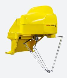
The M-1iA/0.5AL robot has the dexterity of a human hand. This gives it the ability to work in variety of different industries, including the electronics, fine mechanics, medical, pharmaceutical, and food industries.
