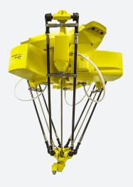
The FANUC M-2iA/3AL is a 6-axis robot made for high speed picking, packaging, and assembly. The advantage of the M-2iA/3AL is that it has a longer reach of 1130 mm with the same 3 kg payload of other FANUC M-2iA/3A models. In addition, the 3 axis wrist helps it to rotate parts when needed and it has a clever design to help make the best use of available workspace.
