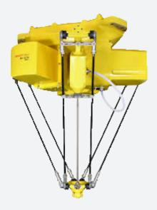
The FANUC M-2iA/3A is a 6 axis delta robot that is built for high speed picking, packaging, and assembly applications. This FANUC robot features an 800 mm reach and 3kg payload; its 3-axis wrist has the freedom to rotate work pieces and tools for assembly.
