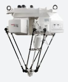
The FANUC M-2iA/6H R-30iB is a high speed picking and assembly "spider" robot. The FANUC M-2iA/6H features 3 axis with no wrist rotation for higher operation speeds. This M-2iA/6H model can handle up to 6 kg and has a +/-0.1 mm repeatability. Advance your pick and place and assembly process today!
