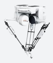
The FANUC M-3iA/6A features 3 rotational axes at the wrist. The FANUC M-3iA/6A is ideal for high speed picking and assembly operations. The M-3iA/6A features a 6 kg payload and can be mounted on the ceiling.
