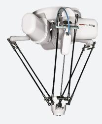
The FANUC M-3iA/6S is a high speed picking robot. The M-3iA/6S is a 4 axis model that features a single axis wrist rotation. This model also includes Visual Line Tracking.
