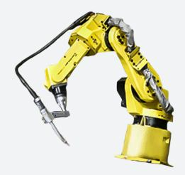
The FANUC ARC Mate 120iB/10LT is a six-axis, overhead rail-mounted robot that provides accurate and consistent path performance necessary for welding and cutting.
