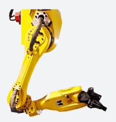
The FANUC M-16iAT is an overhead-mounted robot designed for material handling and machine tending applications. This system features a standard FANUC M-16i R-J3iB robot arm with a modified J1 axis that allows it to be mounted on an overhead rail. Six full axes of motion, one linear and five rotary, allow for greater mobility and the ability to reach a larger work area without sacrificing floor-space.
