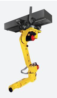
The FANUC M-20iA/20T is the latest rail mounted robot, the lightest model in the range. This M-20iA/20T is a 6 axis machine that is designed to enhance versatility and keep costs down. It can perform a variety of applications including assembly, machine loading, material removal, arc welding, dispensing, and part transfer.
