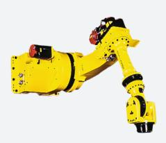
The FANUC R-2000iB/200T is a top mounted robot designed for a variety of applications such as material handling, spot welding, dispensing, part transfer, and palletizing. Delivering precision and speed, the rail mounted R-2000iB/200T is a real space saver on the factory floor and improves machine productivity, up to 30 percent. It combines the large work envelope and small footprint advantages of a linear gantry with the dexterity and reliability of an articulated robot.
