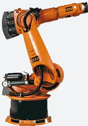
The KUKA KR 360 is a heavy duty robot with a lot of options! This Kuka KR 360 KR C2 arm has a generous payload of 360 kg and a long reach of 2826 mm. The KR 360 Kuka robot can be floor or ceiling mounted to allow for effective use of existing floorspace.
