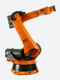
The Kuka KR 210 L has a wider work envelope and a smaller payload than other members of its family. The KR 210 L KR C2 comes in versions approved for foundry or cleanroom use. The cleanroom version meets stringent cleanroom requirements and can be ordered with food-compatible H1 oil. The foundry version is suitable for environments with a high degree of fouling and high temperatures.
