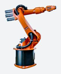
The six-axis Kuka KR 15 is a flexible robot arm that features a light body and medium payload. Flexible and fast, the KR 15 KR C1 is well-suited for handling, assembly, machining, and weldingapplications. The internal components of the KR 15 arm are designed with a straightforward configuration, allowing the arm to remain reliable.
