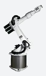
The KR 16-2 CR is the perfect choice for your next cleanroom application. This is a compact, versatile robot that has a 16 kg payload and 1610 mm maximum reach. The KR 16-2 CR provides strength, flexibility, and a solution for diverse applications as it is easily customized. The
