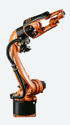
The KR 5-2 Arc HW (Hollow Wrist) is a new type of robot that is considered to be the arc welding specialist. It's attributes truly put it in a class of its own. For instance, it has a 50 mm opening in the arm and wrist to enable the internal routing of the arc welding dress package. This is a huge advantage as it helps to protect the dress package from mechanical influences and whiplash. There are a variety of dress package options available such as torsion-type and infinitely rotating.
