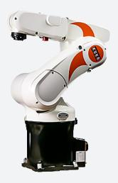
Short cycle times, combined with high accuracy, make the KUKA KR 5 Sixx an excellent choice for many assembly applications. A compact arm with a 5 kg payload, the KR 5 Sixx is available with two reach options: 650 mm and 850 mm. The high-speed arm has six axes and can be mounted on the floor or on the ceiling. A high-performance KUKA PC-based controller makes the KR 5 Sixx KR C2 SR easy to program and operate.
