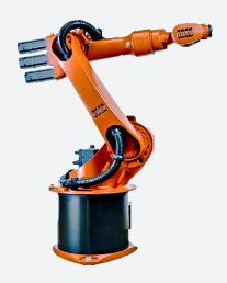
The KUKA KR 6-2 is part of the low payload family. The KUKA KR 6-2 KR C4 robot comes equipped with a KR C4 controller and has a 6 kg payload. Great for many applications, the KUKA KR 6-2 is cost effective and efficient.
