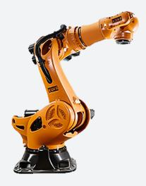
Making palletizing jobs look effortless, the KR 1000 L950 Titan PA can lift up to 950 kg. It offers a long reach, 3601 mm, and is paired with the KR C4 controller which helps to bring versatility by transitioning from hardware-driven to software-driven technology. As a team, the robot and controller make jobs more affordable, efficient, and easier.
