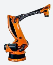
The KUKA KR 180 PA features powerful motors and high-performance gear units. Multiple pallets can be stacked with ease, allowing for fast stacking operations at up to 30 cycles per minute. The mass has been reduced on this arm through the use of carbon-fiber reinforcement. This increases the performance while reducing energy requirements.
