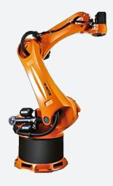
Powerful and robust, yet light and fast, the KUKA KR 300-2 PA palletizing robot will not disappoint. KUKA has designed this robot specifically for high-speed tasks with heavy payloads, up to 300 kg! It has 5 axes, a 3150 mm reach, and is paired with the KR C4 controller.
