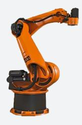
The KUKA KR 300 PA robot can drastically increase your palletizing output. It is well-suited for high speed tasks with high payloads. The result is shorter cycle times and increased throughput.
