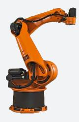
Proven reliable, the KUKA KR 470 PA is the answer to your demanding palletizing needs. This arm features a hollow wrist for cable protection and KUKA components for maximum performance.
