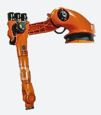
The KUKA KR 150 K is a six axes, 110 kg payload, shelf-mounted robot. The KR 150 K KR C2 is ideal for a variety of applications such as spot welding, material handling, machine tending, and plasma cutting.
