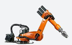
Shelf-mounted robots, like the KR 16-2 KS, offer the customer a greater depth of working envelope in the downward direction. They also have a lower overall height, when compared with the standard K models. These benefits help in certain tasks such as the loading and unloading of machines such as injection molders. The KR 16-2 KS combines all of these beneficial attributes and uses them to also produce reduced cycle times in machine tending tasks.
