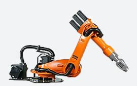
KUKA's KR 16 KS-F is a shelf mounted industrial robot designed for a wide variety of applications such as handling, packaging, cutting, and painting/enameling. Designed with a 16 kg payload and a maximum reach of 1801 mm, the KR 16 KS-F KR C2 weighs 235 kg.
