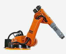
The KR 30-4 KS-F is a six-axis shelf mounted robot. When compared with the K model, the KS offers a greater depth of working envelope in a downward direction. This robot can tackle up to 30 kg in payload and has a 2233 mm reach.
