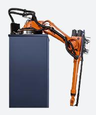
The KR 60 L 16-2 KS is a swift, efficient, and tireless worker that handle up to 16 kg in payload and has a long reach of up to 2952 mm!
