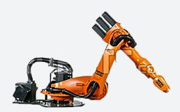
The short stature and deeper 1801 mm reach of this shelf-mounted KUKA KR 6 KS KR C2 model make it an excellent choice for diverse applications.
