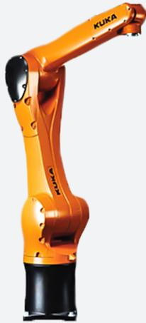
The KR 10 R1100 Fivve (KR AGILUS) is a five axis robot that can provide high speeds and excellent precision for a variety of applications. It is an extremely versatile robot as it requires minimal floor or ceiling space when mounted. The KR AGILUS has a reach of 1101 mm, can conquer payloads up to 10 kg, and is paired with the KR C4 Compact controller.
