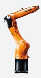
The KR Agilus Sixx R900 is a fast worker, which benefits manufacturers by reducing cycle times and increasing repeatability. The R900 Agilus KR C4 has a compact size, saving space with its small footprint, and also making it very adaptable to several different work environments. Along with being functional, the KUKA R900 Sixx KR C4 compact sets the safety standard, simplifying the human and machine interaction.
