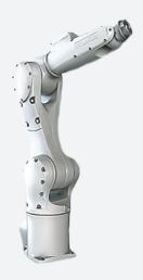
The KUKA KR6 R900 Sixx HM-SC, also known as the KUKA KR Agilus Hygienic Machine, is an extremely clean, fast robot designed for applications involving contact with food or pharmaceutical substances. This robot is hygienic, preventing any contamination happening in your manufacturing process. The KUKA KR Agilus HM robot has a 6 kg payload and 901.5mm reach with an IP67 protection class rating. It is compact and can be mounted on the floor, ceiling, or call.
