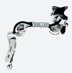
The reversed lower arm of the Motoman MA1650T allows for a large working envelope while conserving floor space. The through-arm cabling is designed to maximize cable life and improve weld performance. The MA1650T DX100 Motoman welding robot cycle times are reduced as a result of using high performance Sigma V AC servo motor control and Advanced Robot Motion (ARM) control.
