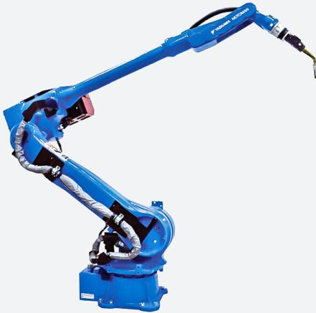
The extended reach of the Motoman welding robot MA3100 provides a way to handle complex arc welding applications. The Motoman MA3100 DX100 robot arm can reach around large parts with quick maneuvers. The ability to wall- or ceiling-mount this arm increases flexibility while conserving floorspace. The MA3100 features the new Sigma V AC servo motor control technology and Advanced Robot Motion (ARM) control. Internally routed cables eliminate cable interference and result in improved performance.
