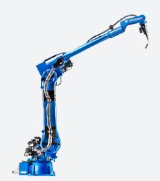
The Motoman MA3120 one of the latest Motoman arc welding robots. With a slim design, this high speed robot has a 6 kg payload, 3121 mm horizontal reach and 5615 mm vertical reach.
