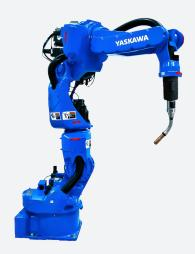
The Motoman VA1400 II is a 7-axis robot capable of high speed arc welding. The Motoman VA1400 II has a streamlined design for better torch access into tight spaces along with improved reach and flexibility. It has integrated through-arm cabling that eliminates cable interference and simplifies programming. The VA1400 II comes equipped with the DX200 controller and can handle a 3 kg payload.
