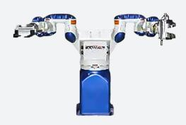
The Motoman DA20 robot offers 13 axes of motion (six in each arm and one single axis for base rotation), resulting in human-like movements. With a 20 kg payload for each arm, the DA20 NX100 is perfect for applications such as assembly, machine tending, packaging, and other material handling tasks.
