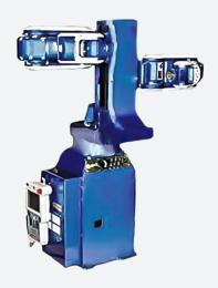
The Motoman DA9IC is a unique dual-arm robot that features coordinated and independent control of up to 11 axes of motion (12 axes with optional linear track). Its compact size, wide working envelope, and internally routed electrical and pneumatic lines make the DA9IC NX100 robot ideally suited to perform multiple processes with small work pieces.
