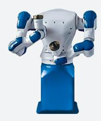
The Motoman DIA10 robot is designed with two arms, each with the capability of handling a 10 kg payload. The arms can work separately, greatly increasing productivity, or they can work together and double their handling ability for heavier tasks.
